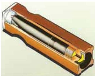
Above: H&K G11 caseless ammunition rifle cutaway.
