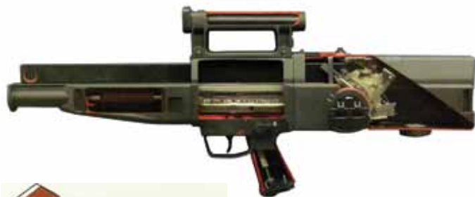
Above: H&K G11 caseless ammunition rifle cutaway.
