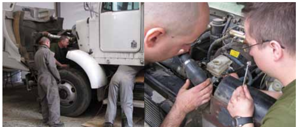
Left photo: Vehicle Technicians from 5 Service Battalion, doing a repair in the accelerator pedal section, clutch and brakes of a truck tractor. Right photo: vehicle technicians connect brake hoses after changing the master cylinder of a Light Support Vehicle Wheeled (LSVW).
