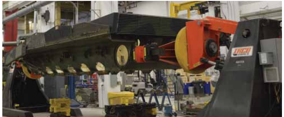
At 202 WD, junior officers have the opportunity to produce new designs and assume full project management, from starting point to submission of deliverables. In this photo, one project junior officers are working on: 360 degrees positioners for a Leopard 2 chassis.
