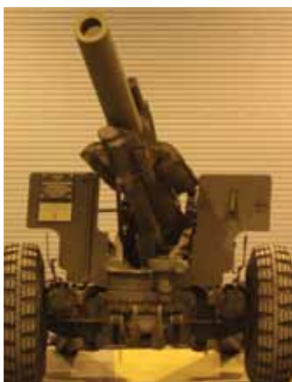
155-mm Howitzer M1A1 Cdn on a Carriage M1A2 Cdn as it was gave back to the city of Barrie.
