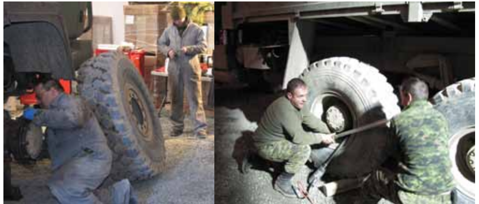
Vehicle technicians from 5 Service Battalion performing different tasks on the axles of Heavy Logistics Vehicle Wheeled (HLVW).
