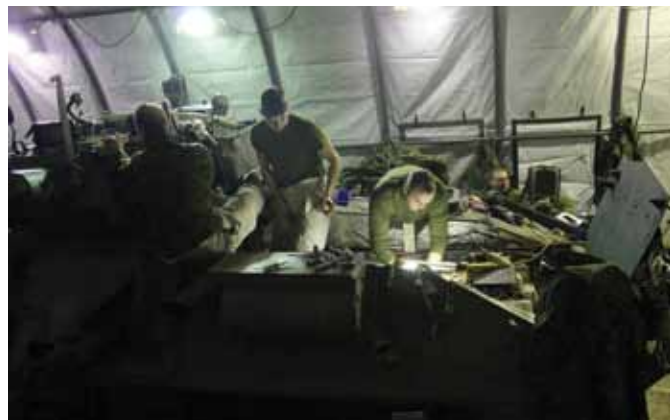
Vehicle technicians changing the engine of a Coyote
