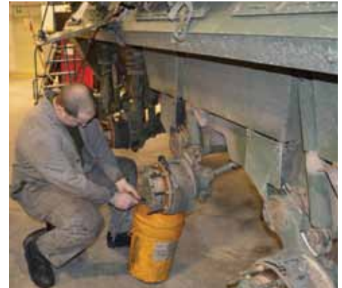
Cfn Rice (Veh Tech) is changing the hub oil on a Coyote.
